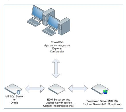
In this configuration, Meridian uses existing DBMS and web servers, and all remaining components are installed on a single dedicated application server.
