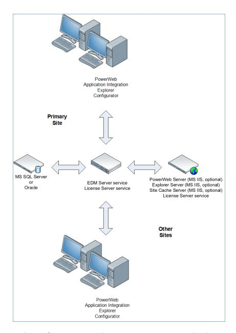
In this configuration, Meridian uses existing DBMS and web servers, and all remaining components are installed on one or more dedicated application servers at each of the organization's sites. Each site hosts its own vaults from which users may work only on documents relative to that site.
