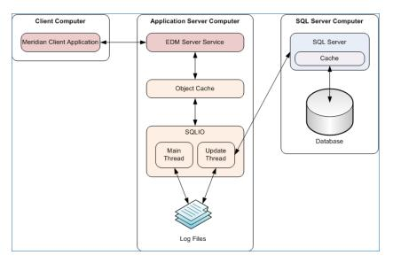
When a Meridian client sends or requests data from the Meridian application server, the EDM Server service communicates with its object cache, which in turn communicates with Accruent SQLIO, which then communicates with SQL Server on the SQL Server computer.
