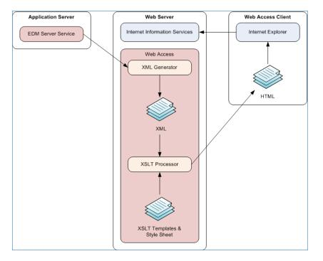
PowerWeb first creates XML files that contain pure data (no presentation) to be exposed by PowerWeb. The XML pages are then converted into HTML. During this step, information about the way the data should be presented on the screen is added. How the information is presented is determined by a set of templates (\*.xsl), which are encoded in XSLT, and a style sheet named amm.css.
