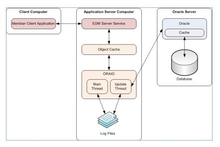
When a Meridian client sends or requests data from the Meridian application server, the EDM Server service communicates with the object cache , which in turn communicates with ORAIO, which then communicates with Oracle on the Oracle server.
